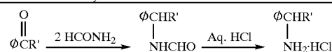
Scheme 6 Literature-based pathway for ready synthesis of a variety of racemic \alpha -substituted benzylamines.
