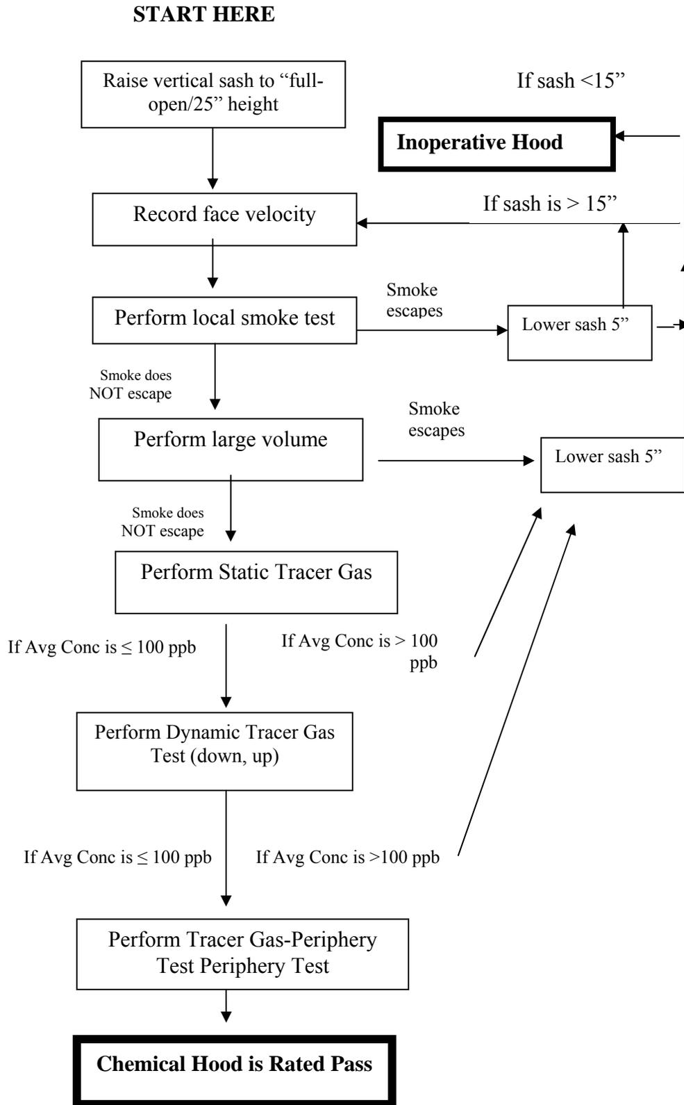
Figure 2: The ASHRAE 110 Test Flow Chart
