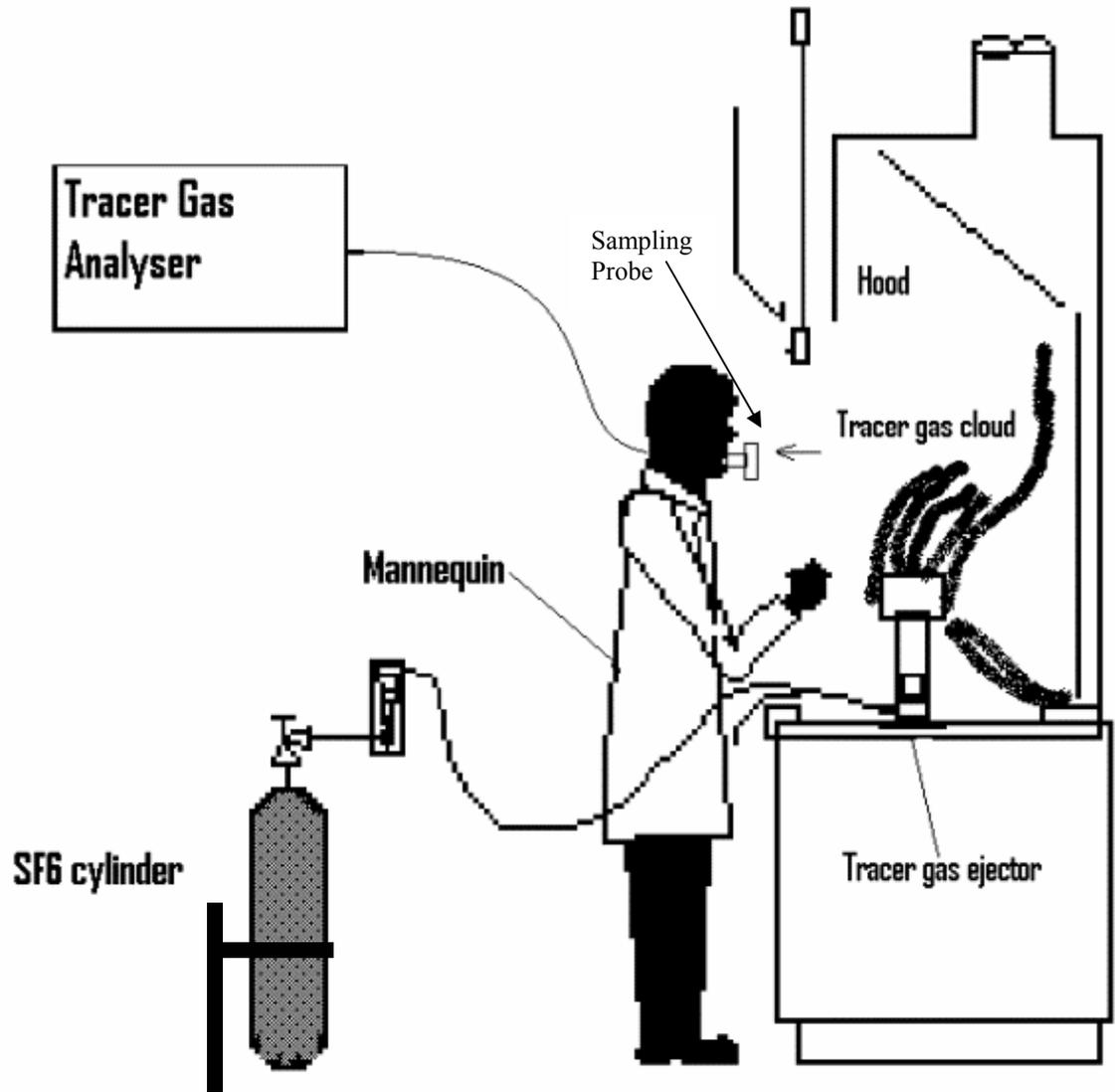
*Figure 1: The ASHRAE 110 Test Setup.*
