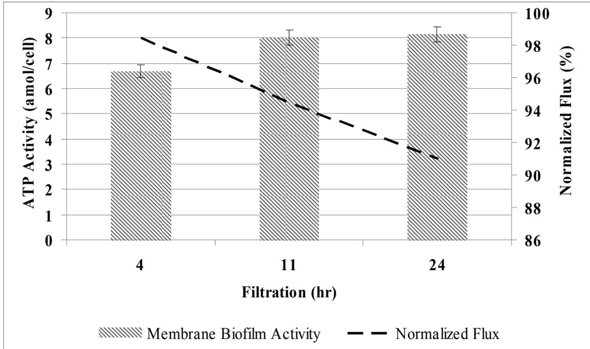
**Figure 3-3(a): Influences of membrane biofilm ATP activity resulted from active *P. fluorescence* biofoulant on the membrane permeate flux during different filtration duration (4, 11, 24 hr). Error bars represent  $\pm$  one standard error of the mean.**
