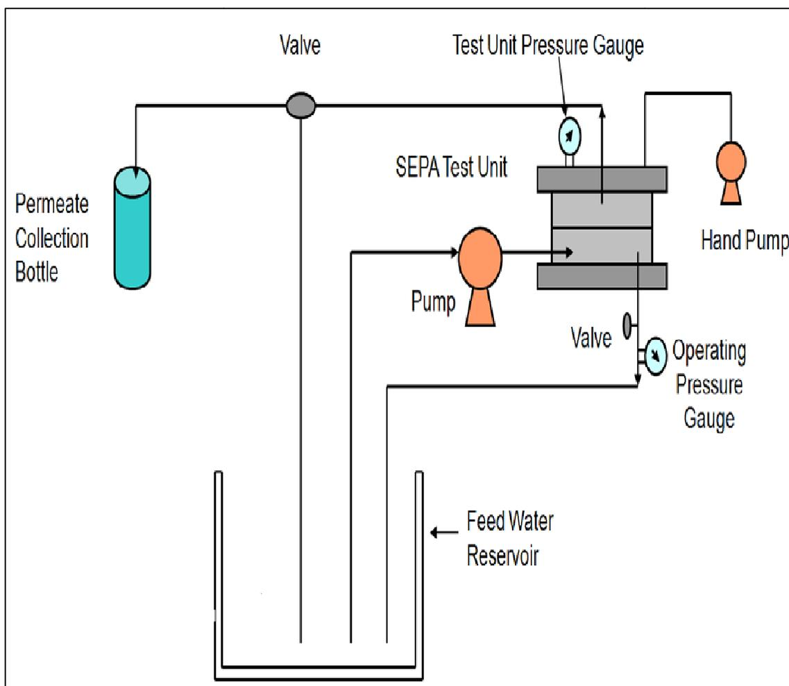
**Figure 2.1: Cross-flow membrane filtration system pumping feed water through UF membrane and circulating concentrated and permeate water in the reservoir. Trans-membrane pressure could be adjusted with the operating pressure valve.**
