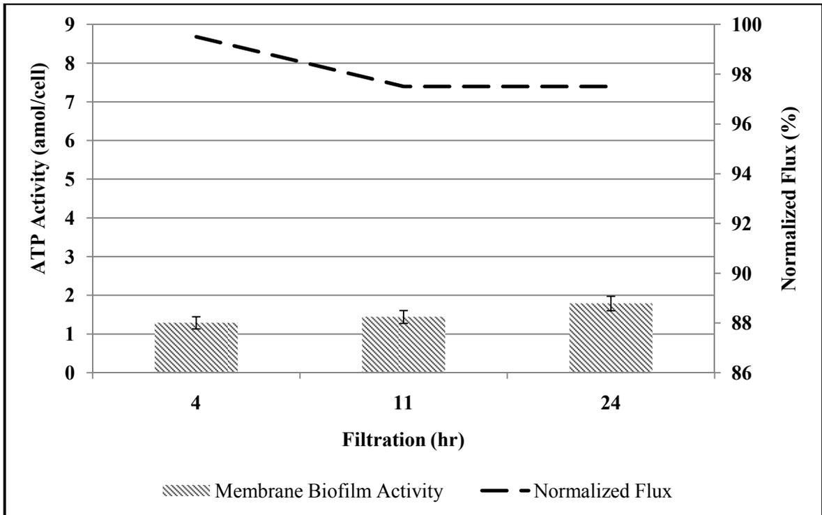
**Figure 3-3(b): Influences of membrane biofilm ATP activity resulted from inactivated *P. fluorescence* biofoulant on the membrane permeate flux during different filtration duration (4, 11, 24 hr). Error bars represent  $\pm$  one standard error of the mean.**
