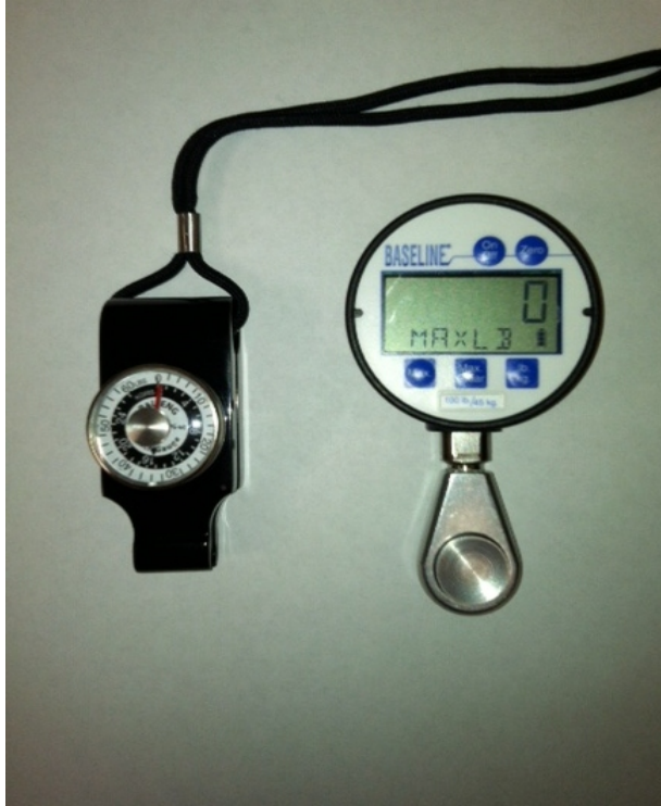
Figure 1. Instruments used in this study. B&L pinch gauge shown on the left. Baseline digital hydraulic pinch gauge shown on the right.
