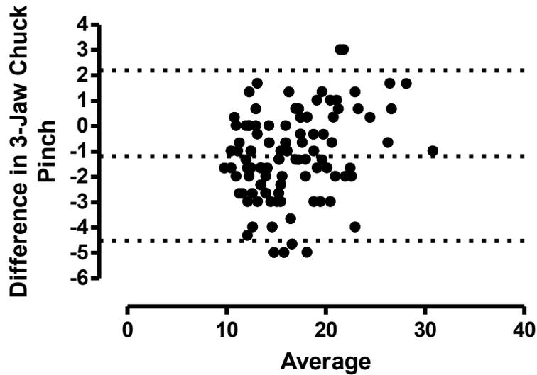
*Figure 3.* Bland-Altman Plot for 3-Jaw Chuck pinch. The difference of mean averages of each participant represents one dot (102 total). Bias=-1.18; SD=1.70. 95% confidence intervals (CI) shown in top and bottom dashed lines (-4.52, 2.17). Most participants fell between the confidence interval and no trends were seen among differences in mean averages.
