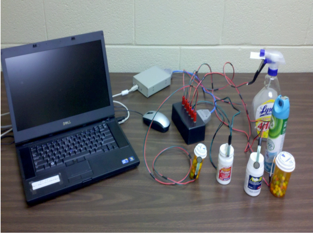
Figure 1. Containers with sensor placements
